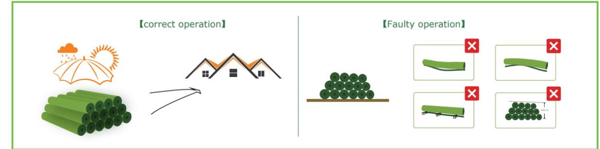
**Note :** The artificial turf shall be stored in ventilated, dry, and pollution-proof warehouses, preventing from direct sunshine, rain, moist, fire, chemicals, and over-extrusion.
